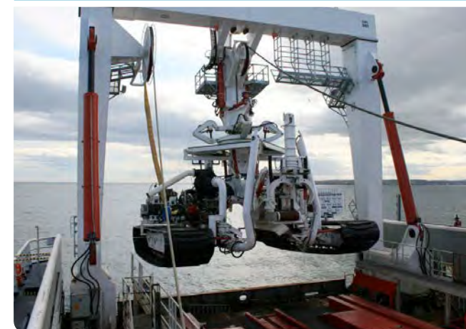
Figure 2-10 i-Trencher chain trenching vehicle & LARS
