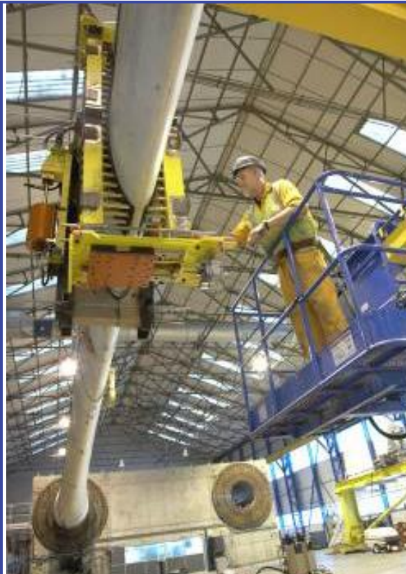
Figure 4.2.7 The blade testing facility at Narec.
