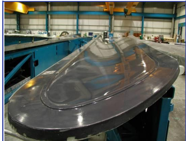
Figure 4.3.1 Wind turbine blade mould.
